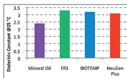
Figure 2 Dielectric Constants of Four Liquids
