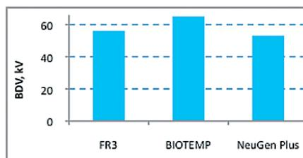
Figure 1 Average AC Breakdown Voltages (BDV) for Three Natural Esters (ASTM 1816, 2 mm gap)
