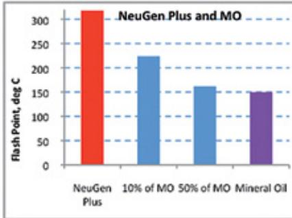
Figure 13 Flash Point for Mixtures and Non-Mixed Liquids
