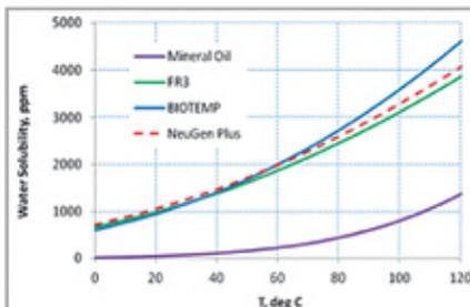
Figure 8 Water Saturation Solubility of Four Liquids vs. Temperature
