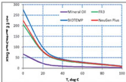
Figure 7 Kinematic Viscosity of Four Liquids vs. Temperature
