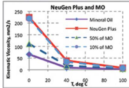
Figure 15 Kinematic Viscosity for Mixtures and Non-Mixed Liquids
