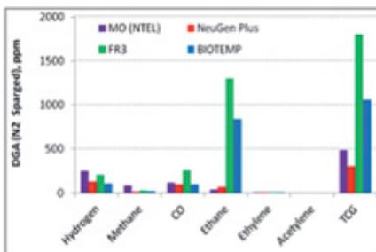
Figure 6 Stray Gassing Results under Nitrogen Sparging Conditions (ASTM D7150)
