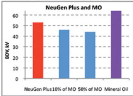
Figure 12 AC Breakdown Voltages (BDV) for Mixtures and Non-Mixed Liquids
