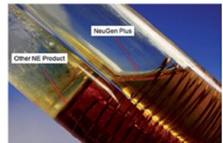
Figure 11 NeuGen Plus and Other Natural Ester Fluid after Testing at 120 °C with Oxygen
