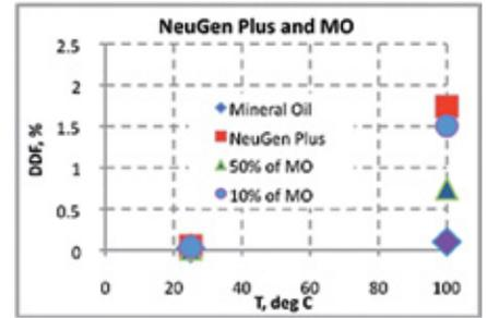
Figure 16 DDF for Mixtures and Non-Mixed Liquids
