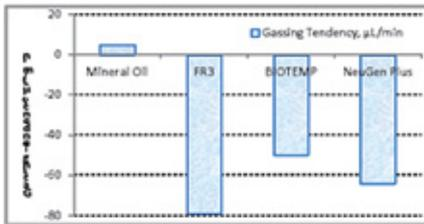
Figure 4 Gassing Tendency of Four Liquids at 80 °C under Electrical Stress (ASTM D2300)
