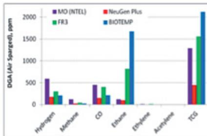
Figure 5 Stray Gassing Results under Air Sparging Conditions (ASTM D7150)
