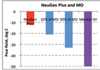
Figure 14 Pour Point for Mixtures and Non-Mixed Liquids
